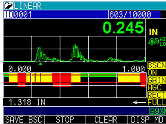
Split A-scan, B-scan with live parameter adjustments
