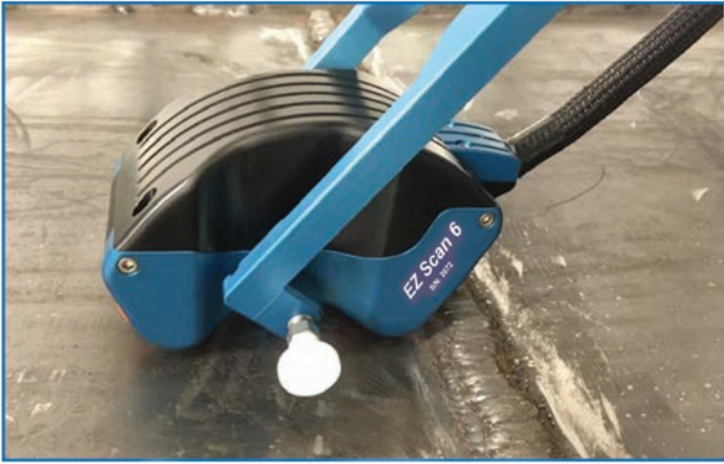
Easily scans over welds
