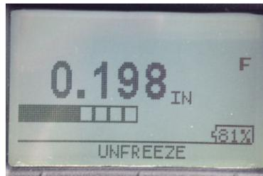
To take thickness readings, simply apply a small amount on fluid (couplant) to the test object and firmly hold the transducer on the part. You will see a number appear on the display and the quality bar fill up from left to right and become solid as the reading becomes more stable.
