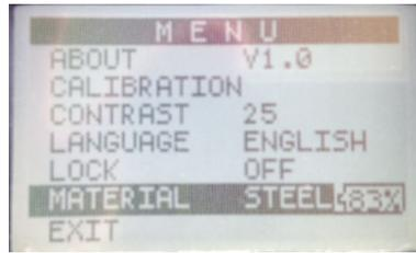
From the Menu/OK, scroll up or down to Material, press Menu/OK to see available materials. The gage defaults to first power on and upon re-set to Steel .2330 IN/Usec. If there is a star next to the velocity, it means that the velocity has been changed manually or via the calibration process. When making measurements on various materials, it is recommended you begin with the one closest to the material you are trying to measure.
