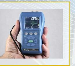
Danatronics introduces the first ever hand held ultrasonic precision thickness gages with COLOR A-Scan. The UPG-07DLCW is a hand held ultrasonic precision thickness gage designed to non-destructively measure most engineering materials with the greatest thickness range. So if you are measuring coil steel, fiberglass thickness on boats, titanium golf club heads, plastic bottles or even rubber tires . . . put us to test, we measure up.
