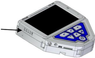
Fig. 15: openings for adjusting the monitor settings
