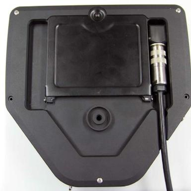
*Fig. 9: Camera cable fed through guide*
