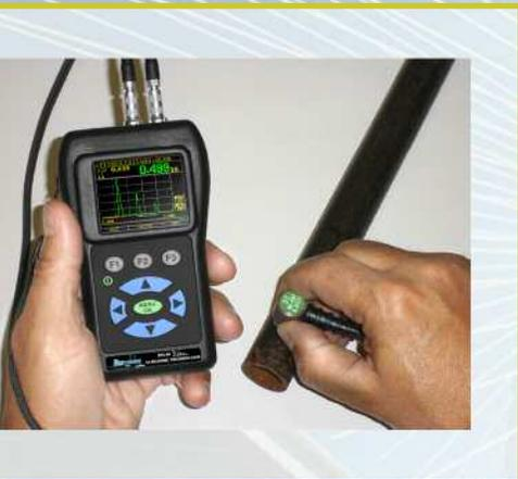
With more than 75 years of world-wide experience in Ultrasonic designs, Danatronic is proud to pioneer the world's first hand held ultrasonic thickness gage with color display; our EHC09 color wave series. Unique features include live **COLOR** A-Scan, B-Scan, 100K thickness reading (3500 waveforms) datalogger with interface program, vibration and **COLOR** change of waveform on alarm.
