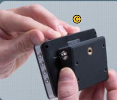
(C) Once aligned, press display down until display locks into wedge mount.
