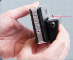
NOTE: Do not force alignment. Be certain display is right side up, "ON" button on top right.
